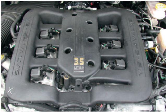
Figure 2.331 Six direct ignition coils in position
